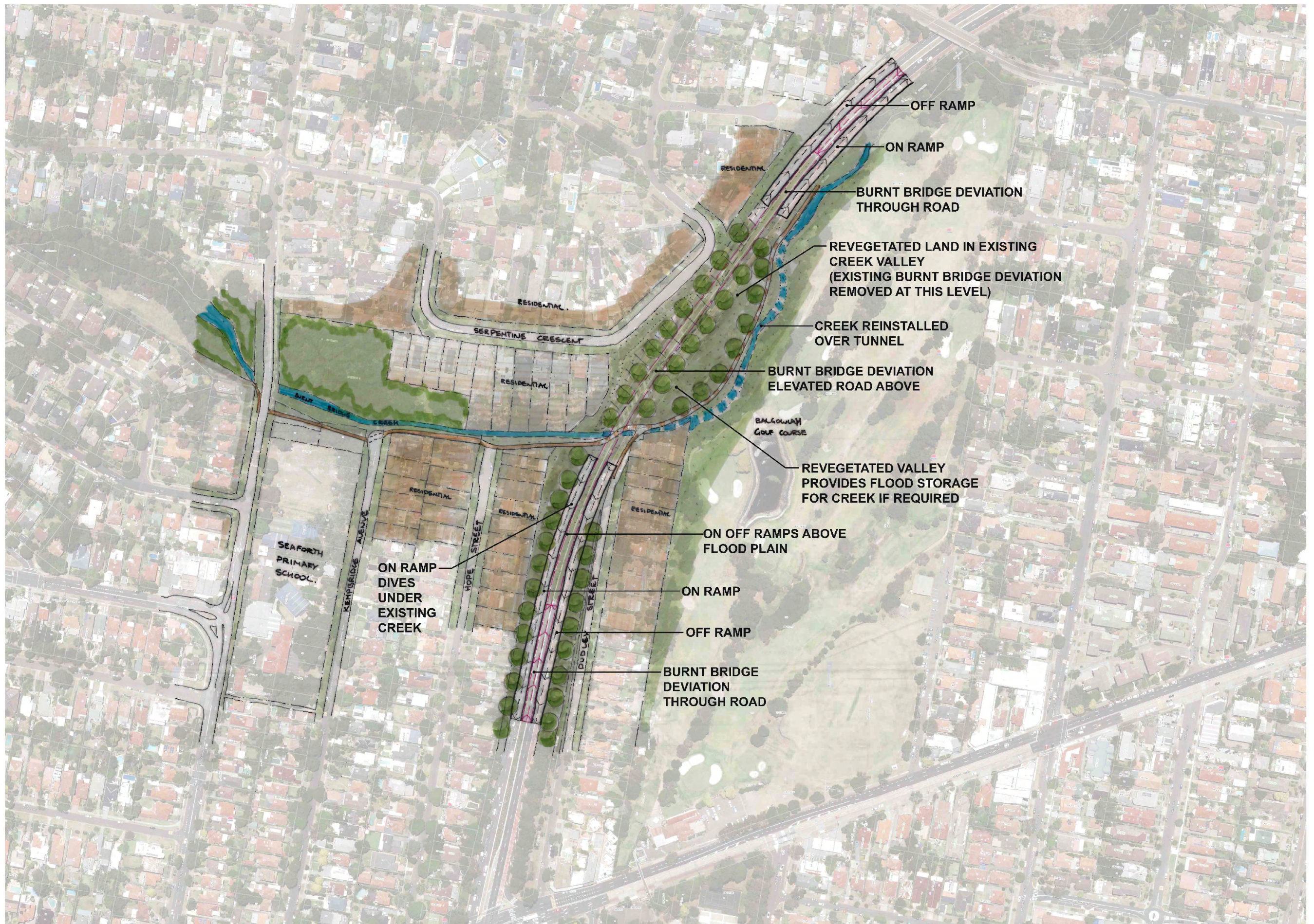
ALTERNATE OPTION- BALGOWLAH TUNNEL PORTAL (GROUND SURFACE LEVEL)
